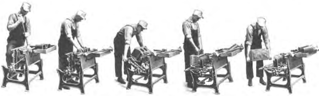
Figure 1. Process of block-making from Sears's Concrete Machinery, Specialty Catalogue, 1917, p. 15, Sears, Roebuck and Co. This is the downface type machine that H. S. Palmer invented.
