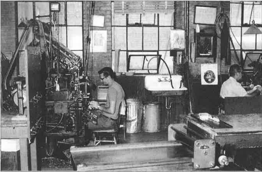
Skilled operators set lines of lead type on these Linotype machines in this photo taken in the 1960s. The device with the rollers in the foreground is a proofing press, used to print copies of stories for proofreading.
