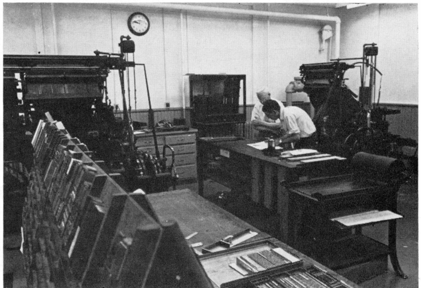
Separate rooms for the major shop functions are a feature of the new facilities for the Journalism Laboratory Press. This is a view of the composing room and its linotype equipment.
