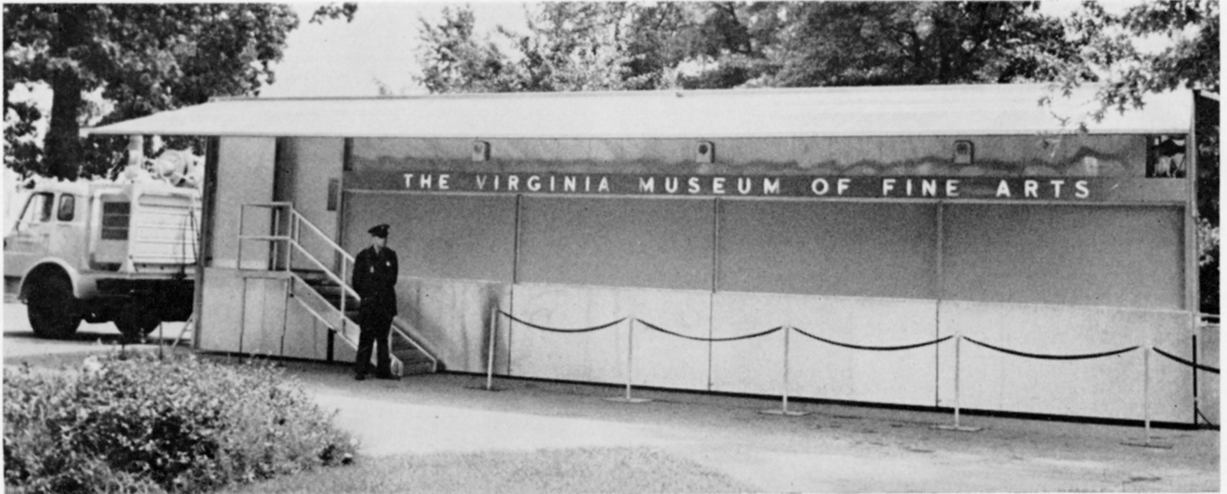
Artmobile IV, the Virginia Museum's "collegiate artmobile," is displayed in Richmond prior to embarking on its first tour of Virginia campuses in the fall of 1966. Display panels on the outer walls are revealed when built-in hydraulic lifts raise the sidewall-awnings. The interior is outfitted with rubber tile floor, accoustical tile ceiling, monk's cloth walls, air conditioning, humidity controls, and elaborate fire and burglar alarm systems.
