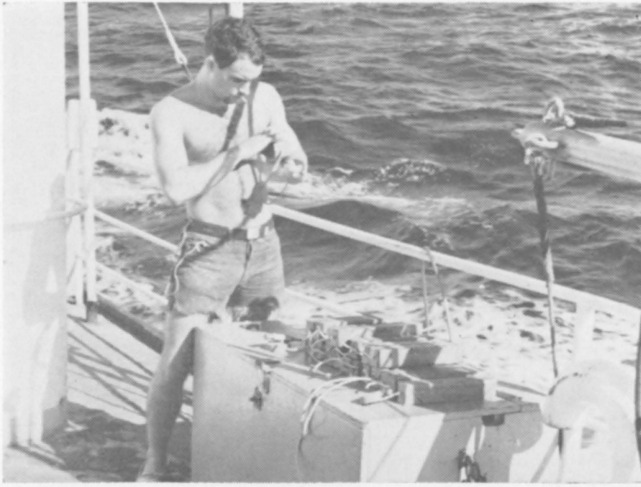
CHIP ROADMAN, Washington and Lee senior who accompanied the author on the oceanographic voyage, is shown lighting fuses for depth charges in the Vema's seismic refraction research program.
