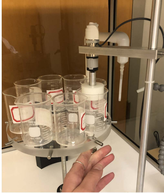
Figure 2.2: This image shows our dipping machine, StratoSequence VI by nanoStrata Inc. in use. The jars are oriented in the machine such that they are dipped in PDDA, rinsed in DI water, dipped in nanoparticles, and rinsed in DI water again.
