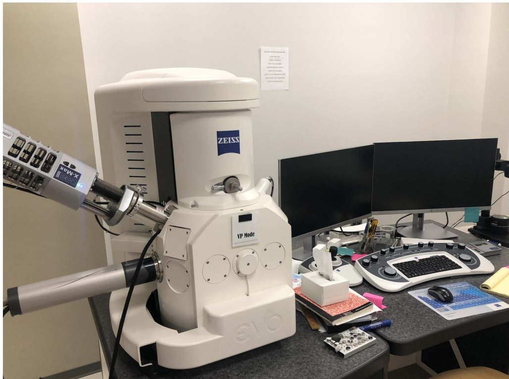
Figure 1.6: Set-up of an SEM. The sample is placed inside the chamber seen on the left-hand side of the photo, and the image can be seen on the monitors seen on the right-hand side of the photo. The image is focused, zoomed in, and adjusted using the knobs on the keyboard.
