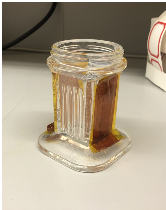
Figure 3.5: Parallel-plate capacitor made of copper tape across a staining jar, with field oriented perpendicular to the slide. The yellow tape is insulating tape to ensure safety due to the high voltages being applied across the capacitor
