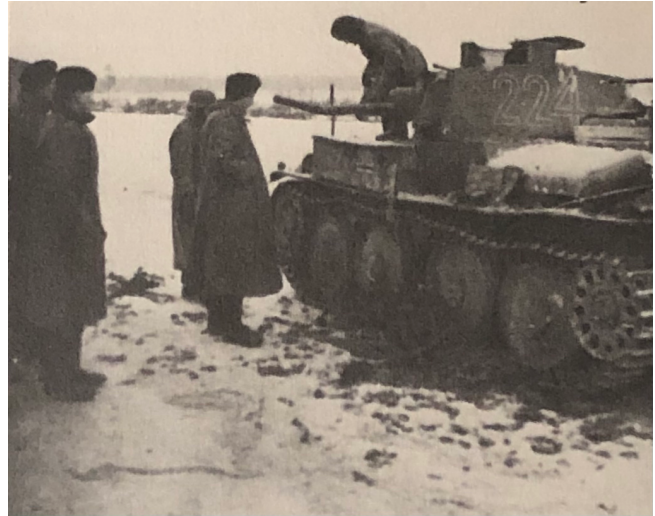
Figure 4: Fuchs' wrecked tank after the skirmish of November 21 st . Fuchs' Wehrmacht 38t tank was far from the only German tank to meet its match in Russia. Early-war tank models, such as the 38t, would prove to be quite vulnerable when in combat against Soviet tanks and infantry armed with anti-tank guns due to their relatively thin armor in comparison to their Soviet counterparts.
